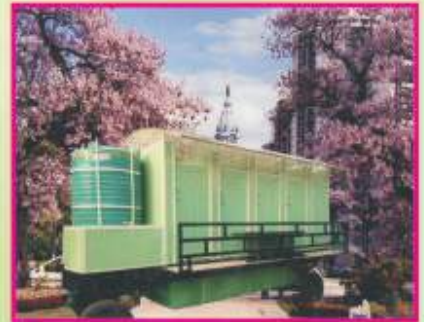
4 Tyre mounted 10 Seater Mobile Toilet Van with lower Tank
